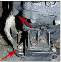
The positive solenoid wire is easily identified in that it is connected to the solenoid by means of a push-on style connector.
